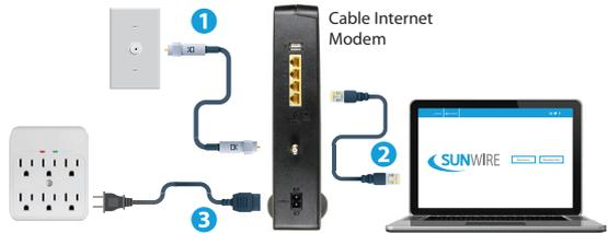
1. Connect the coaxial cable from the wall outlet to the coaxial connector on the back of the modem (hand-tighten to avoid damaging connectors). Contact Sunwire if you cannot find the wall outlet.
